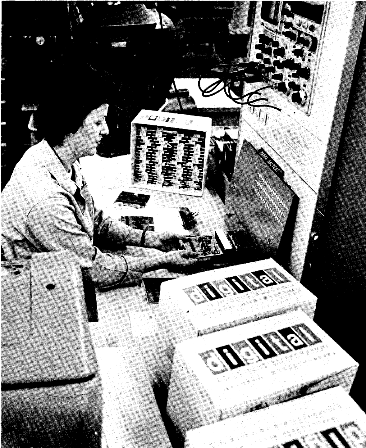
To insure reliability, a wide variety of dynamic tests are performed on-line by a computer controlled system.
