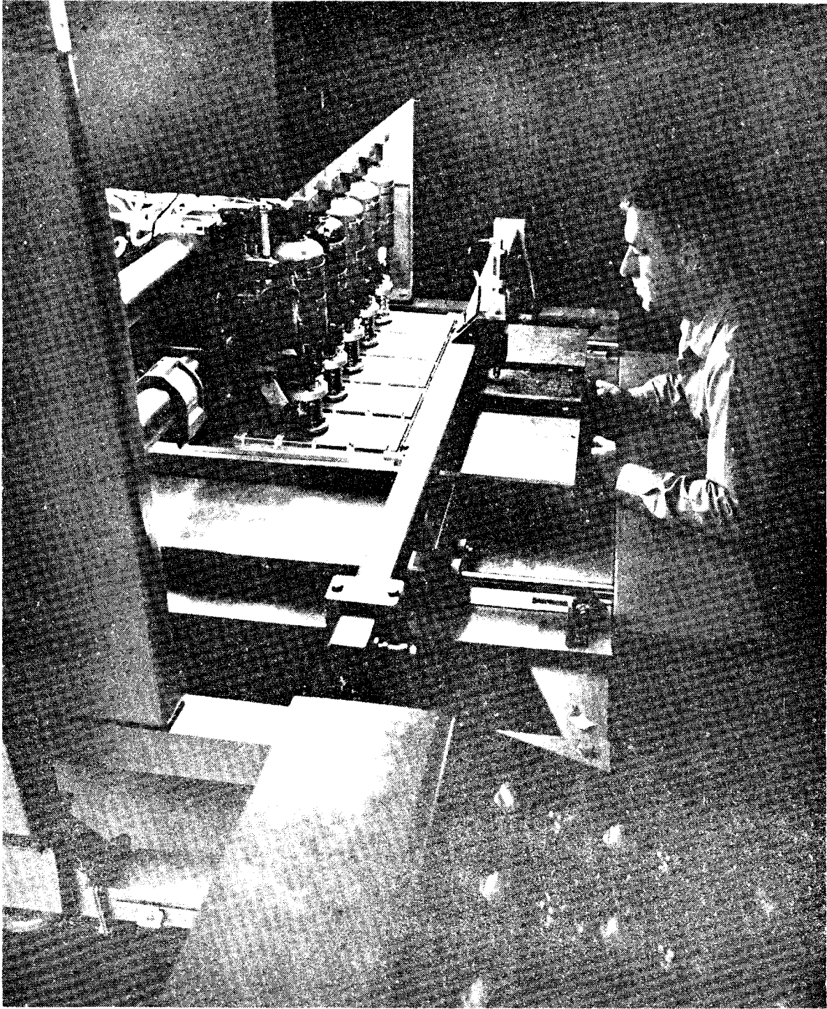
Ten spindle automatic machine drills 40 boards simultaneously, provides precision component layout.
