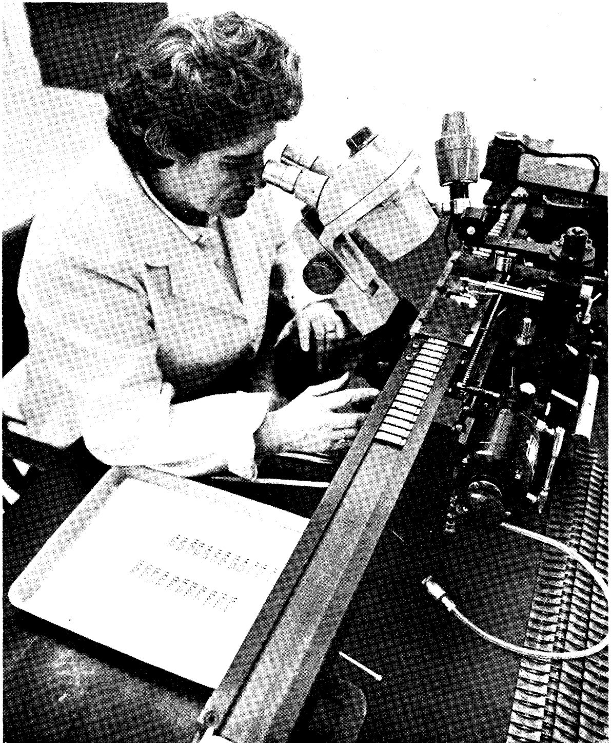
Thermal compression bonding ties semiconductors into hybrid networks.
